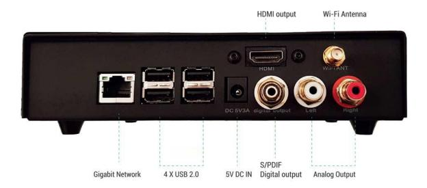
**GIGABIT NETWORK:** Wired Network interface. This is the suggested network connection for playing Hi-Resolution material. Connect this interface to your router via an Ethernet cable.
